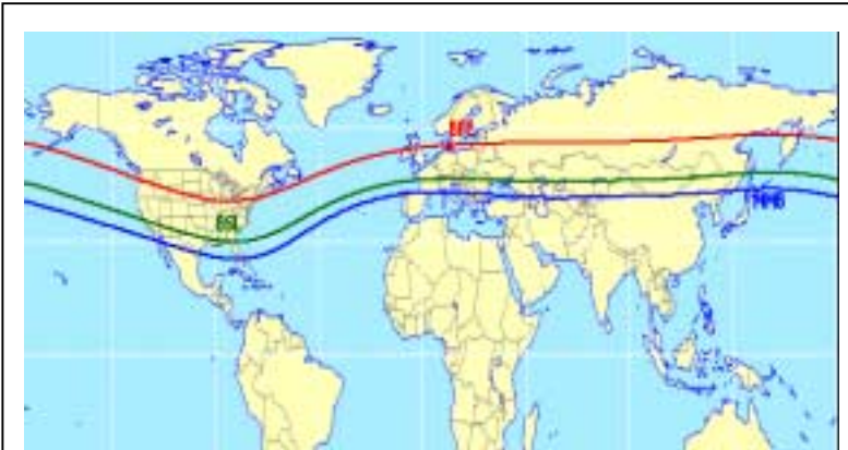
Figure 2: Large rate of change magnetic field disturbances (dB/dt in nT/min) observed during the March 13, 1989 storm were extensive and illustrative of a large storm. The largest dB/dt observed occurred at a Danish magnetic observatory BFE with a 2000 nT/min rate of change of local magnetic field. This Iso-Telluric chart describes equivalent locations worldwide had the same 2000 nT/min impulsive disturbance occurred at other local times (as shown in red). The locations depicted would follow the geomagnetic latitudes rather than geographic latitudes, hence the large low-latitude excursion over North America. For perspective the level of dB/dt that precipitated the Hydro Quebec collapse was only 400 nT/min. Levels this high were observed at very low latitudes, which would encompass most of North America and Europe (as shown in green). Levels of 200 nT/min can easily produce significant power system impacts which for this storm extended to even lower latitudes (as shown in blue).
